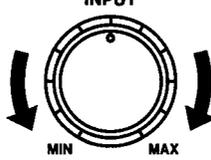
Adjust the recording level so that the peak level meter is between "◆" and "0".
