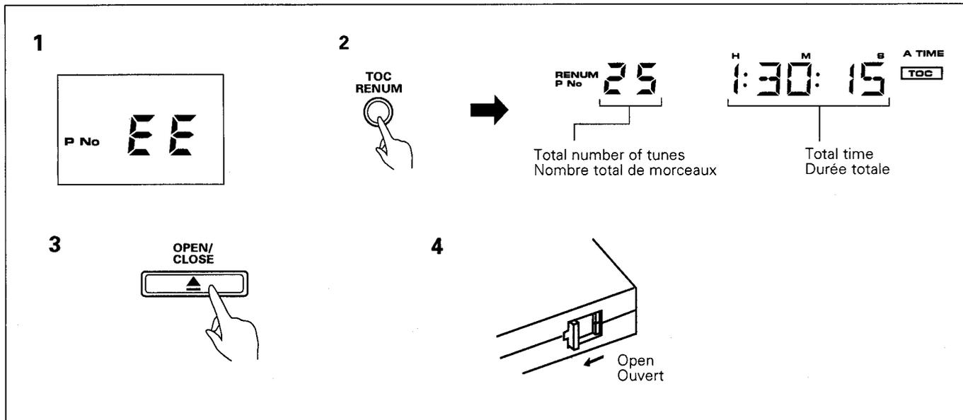
**1 Before writing the TOC, make sure "EE" is displayed.** "EE" is displayed immediately after the End Mark is recorded after recording is completed. Or, load a cassette and press ►► and wait until the end search operation is completed.
