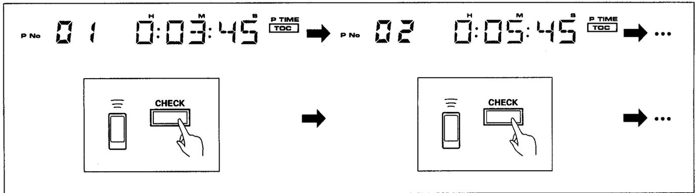
Press CHECK. Each time CHECK is pressed, the display changes as shown.
