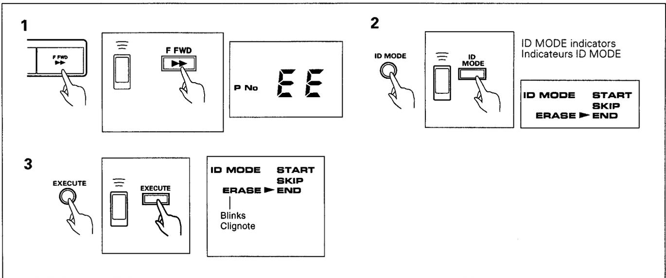
The End Mark is automatically erased when you carry out an end search operation and then continue recording from the end position. However, you can also erase an End Mark using the following procedure.
