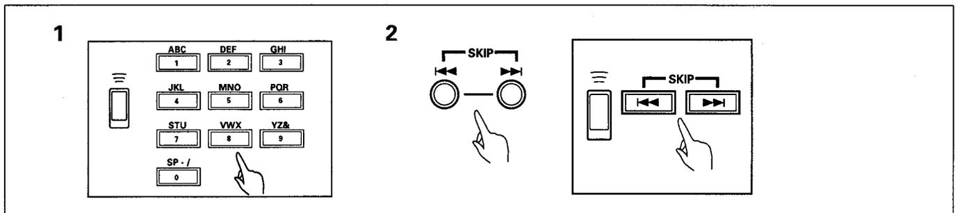
This function enables you to skip a desired number of tunes (up to 9 tunes) forward or backward and start playback from that location. Tune skipping is possible in stop mode, during playback, and in pause mode. If carried out in pause mode, the unit will re-enter pause mode after locating the designated tune.
