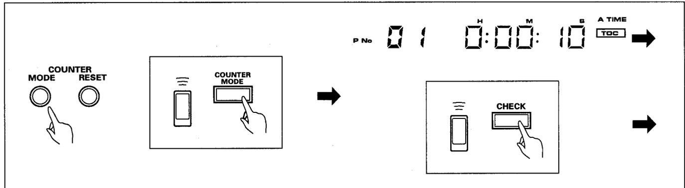
While the length of a tune is displayed, press COUNTER MODE to display the A-TIME. Now, each time CHECK is pressed, the start time of each tune is displayed.
