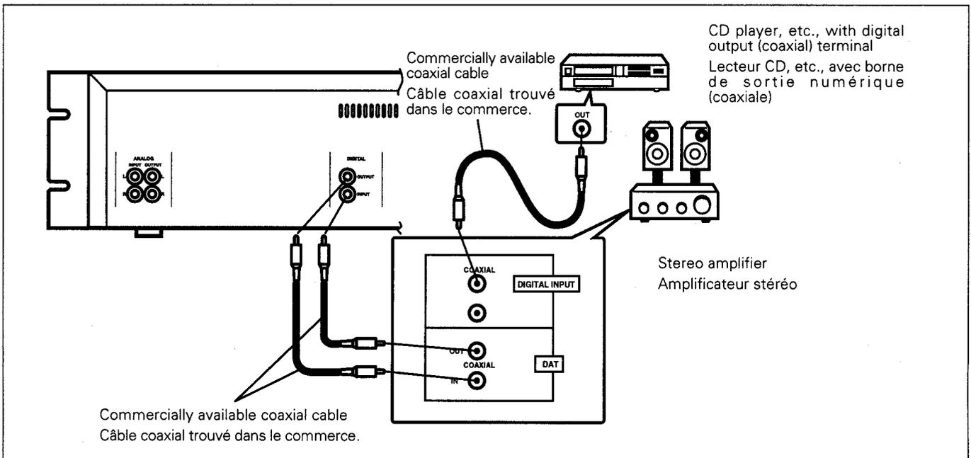
Set the front panel's INPUT selector button to "COAX". "COAX" appears in the upper right corner of the display.
